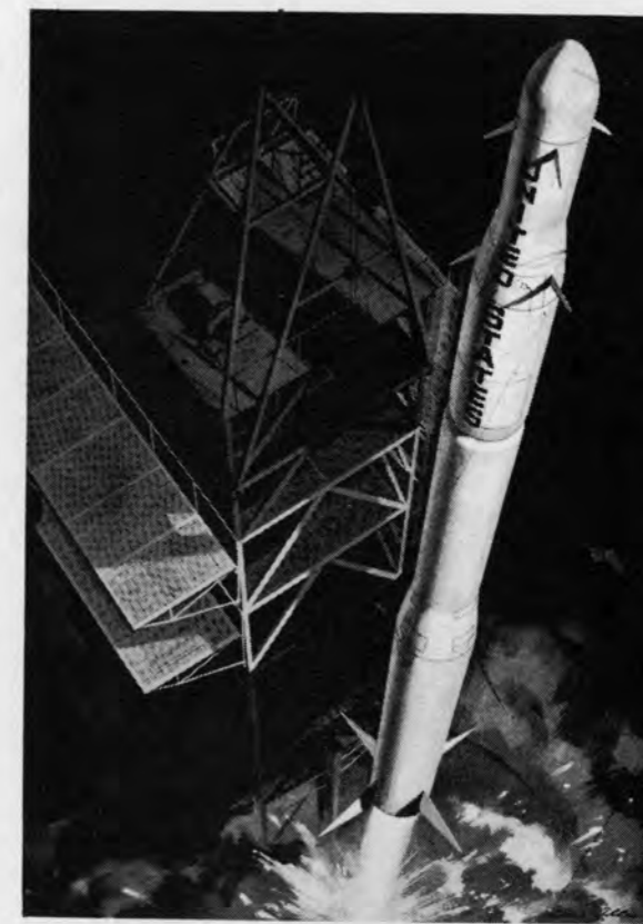
FUTURE SPACE TRAVELER. Scheduled to do much of NASA's research in space is Scout . Vought Astronautics has a contract for the development of this 4-stage research rocket and its 7-story launcher.
